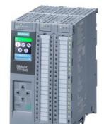
\*\*\* Spare part \*\*\* SIMATIC S7-1500 Compact CPU CPU 1511C-1 PN, central processing unit with work memory 175 KB for program and 1 MB for data, 16 digital inputs, 16 digital outputs, 5 analog inputs, 2 analog outputs, 6 high-speed counters, 4 high-speed counters for PTO/PWM/frequency output 1st interface: PROFINET IRT with 2-port switch, 60 ns bit performance, incl. push-in front connector, SIMATIC Memory Card required
