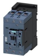
power contactor, AC-3 80 A, 37 kW / 400 V 1 NO + 1 NC, 230 V AC/50 Hz 3-pole, 3 NO, Size S3 screw terminal
