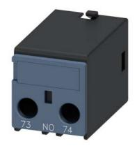
auxiliary switch, on the front, 1 NO, 73/74, current path: 1 NO, cable entry from below, screw terminal, for contactors 3RT2 and contactor relays 3RH2
