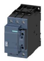
capacitor contactor, AC-6b 50 kVAr, / 400 V, 3-pole, 220 V AC, 50/60 Hz, auxiliary contacts: 1 NO + 1 NC, screw terminal, size: S2  $\,$
