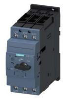
Circuit breaker size S2 for motor protection, CLASS 10 A-release 28...36 A N-release 520 A screw terminal Standard switching capacity
